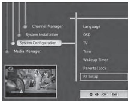
3. Press the ▲▼ buttons to choose the options and then press the ◀▶ buttons to adjust the settings.
