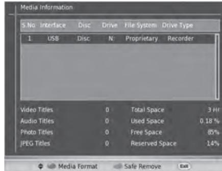
3. When you press the **RED** color button a confirmation will be displayed and press the **◀▶** buttons to select **Yes** and press the **OK** button to Format Hard Drive and the "Media formatted Successfully" message will be displayed. If press the **◀▶** buttons to select **No** it will return to the previous menu.
