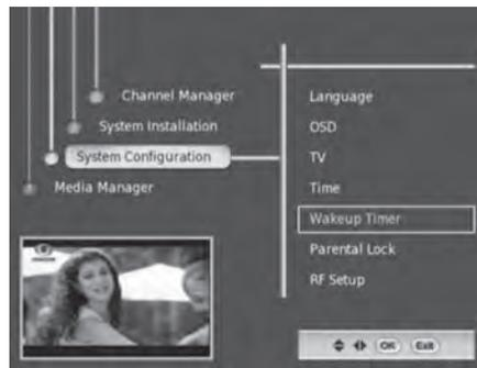
2. Press the ▲▼ buttons to select **Wakeup Timer** and then press the **OK** button to display the menu.
