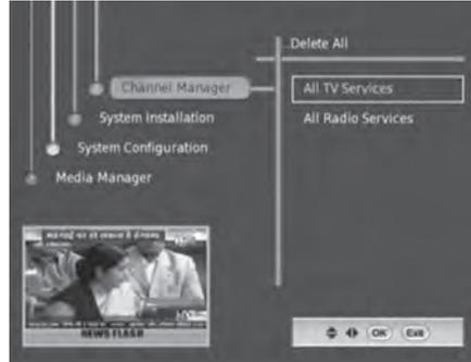
3. Press the **▲▼** buttons to select **All TV services** or **All Radio services** and press the **OK** button to confirm and then the password entry dialog will be displayed. (Default password is 0000)
