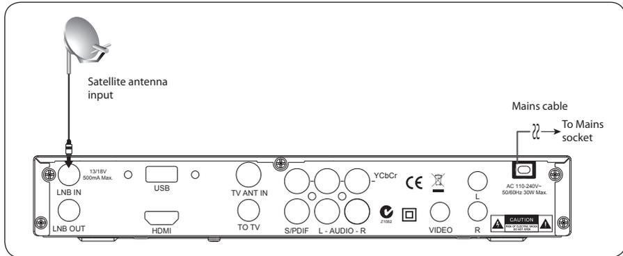
Connect mains plug last, ensure your receiver is connected to the TV and Dish before plugging in to mains power.
